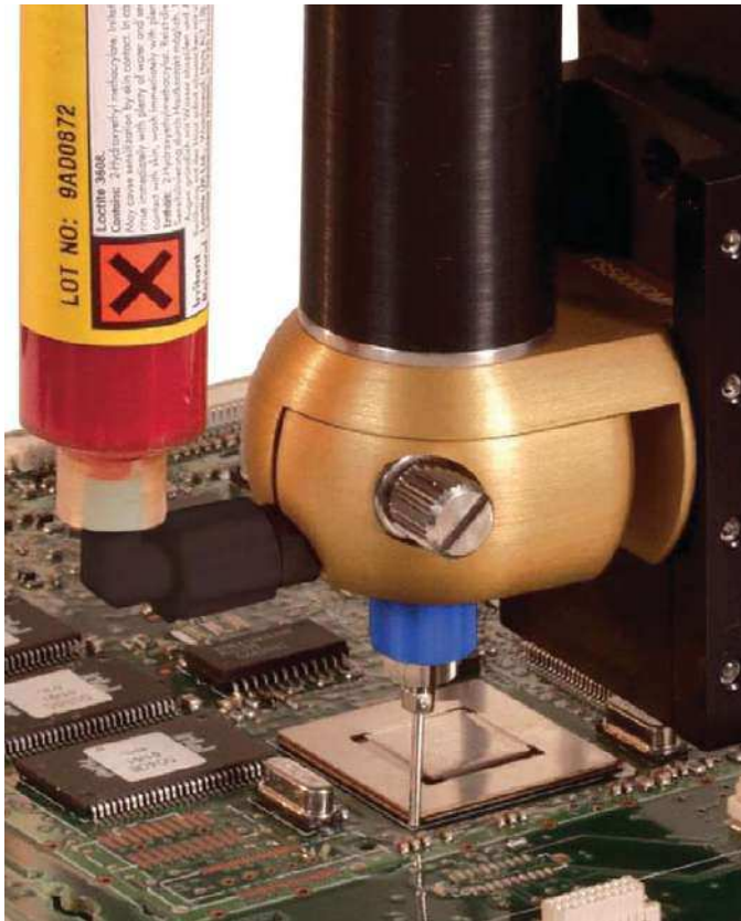
TS5000DMP - Performing underfill
