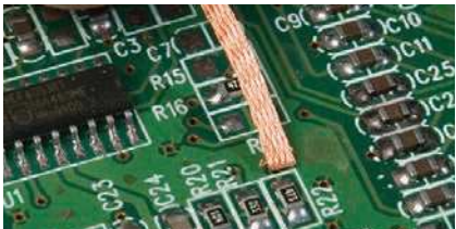
Match braid width to contact area
